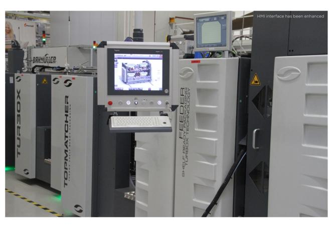
Specified for running small products and shelf ready packaging, the BTX 1450/1700 is equipped with the well-known two-bay Topmatcher.
