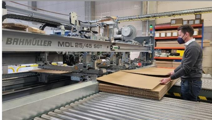
Manfred Sarow is enthusiastic about how productively XXL boxes can be produced on his new line. Stitching, gluing and taping with the servo driven TopSpeedTaper. Gluing is possible in combination – cold and hot melt. A real innovation for semi-automatic lines.
