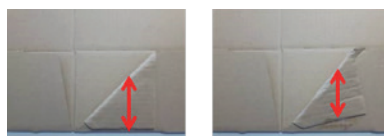
Different diagonal length of folded and misfolded flap
