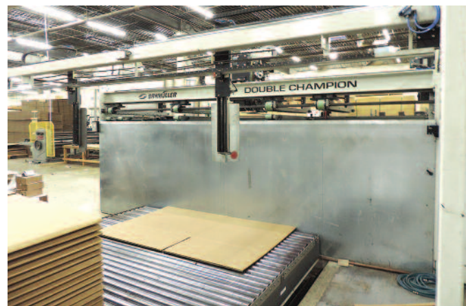
The oscillation stitching head on Ox Box's Double Champion operates at a speed of 850 stitches per minute. It stitches and glues a variety of two-piece corrugated boxes.
