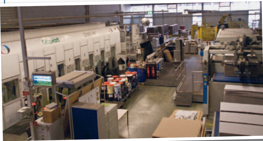
A six colour Gopfert Ovation, equipped with JB dryers, feeds a Bobst Mastercut die-cutter. Below: The Uniqueject ejects defective boxes onto a lower out-feed conveyor.
